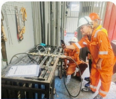
Hydro Test of Fire Extinguisher
