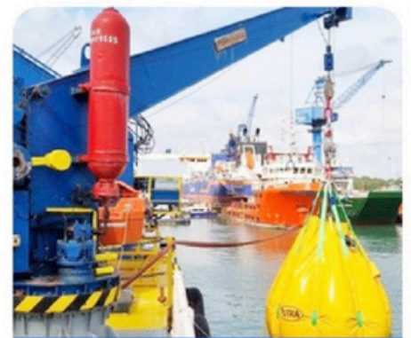
Load test of Rescue boat davit
