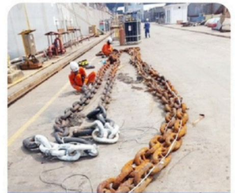
Chain Sling Inspection
