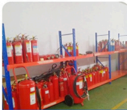
Fire Extinguisher after service
