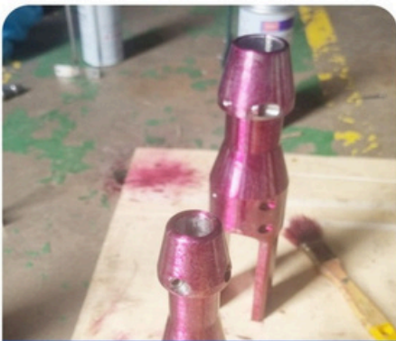
Penetrant Test Socket
