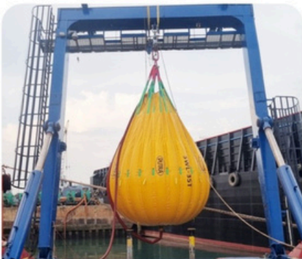
Load test A- Frame
