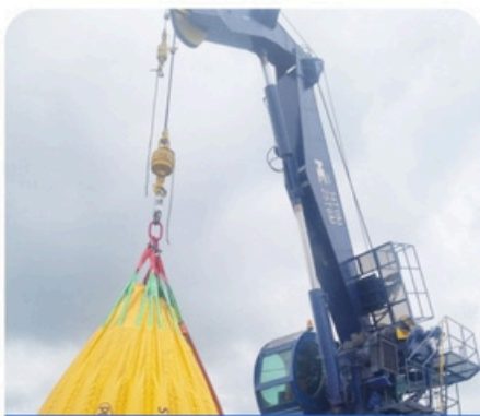
Load test Knuckle Crane
